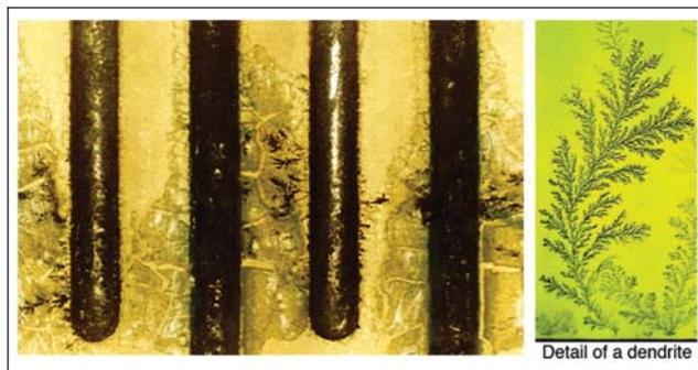
**Figure 3-1 Dendrites Grown Between Oppositely Biased Conductor Lines**
